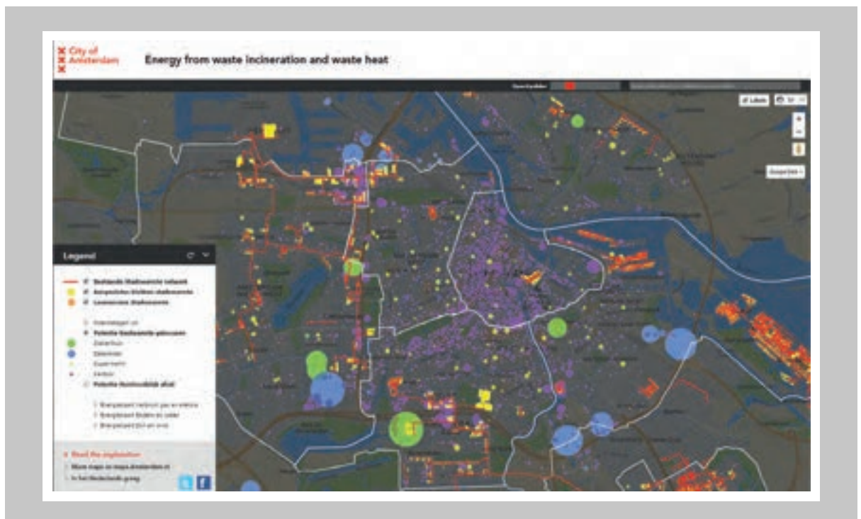
Ill. 53: Energy atlas of Amsterdam, district heating network supply, waste heat and waste potential
