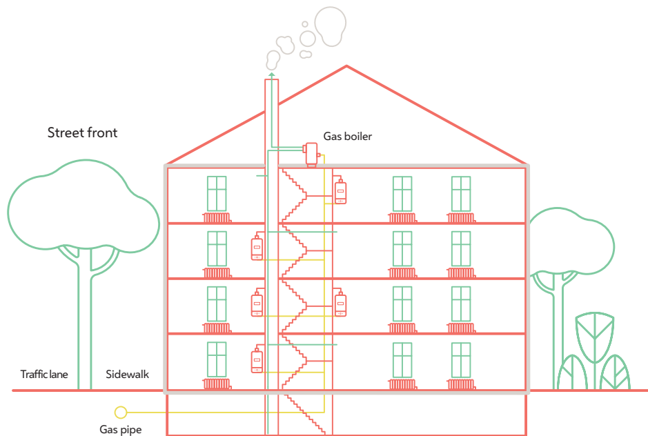
Figure 17 Shared gas boiler as an interim solution.
